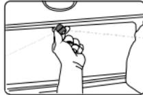
4. Insert camera wire through newly drilled hole and mount securely in place.
