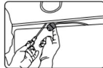
6. Fix the second screw and tighten both screws.
