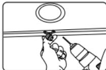
2. Attach tape to the bracket of the camera, and drill a small hole for the first screw.
