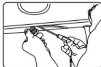
3. Use a screw driver to fix the first screw, but don't tighten it yet.
