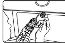
5. Mark the position suitable for the second screw and drill a small hole for it.
